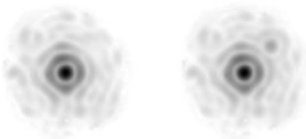
Figure 2. Left: experimental PSF in K band; the Strehl ratio is about 40%. Notice the diffraction pattern and the irregular structures in the halo. The PSF has been oversampled for a visualization purpose: the FWHM of the peak in the original frame is \sim 3.6 pixels. Right: simulated binary star given by the superposition of two copies of the PSF with a flux ratio of 20 and a separation of \sim 0.5 arcsec. It is evident that in order to analyze the fainter component it is necessary to take into account the halo contamination of the brighter one.
