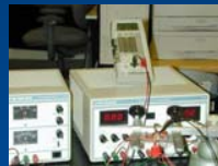
Figure 2: DC Power Supply used to test prototype
