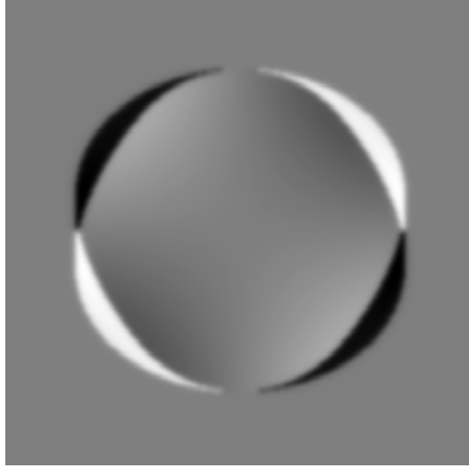
Figure 16. Simulated curvature sensing difference image corresponding to the pure Zernike term Z_{4,-2} for a circular aperture. It is easy to distinguish the zeroth order boundary image from the first order interior image.
