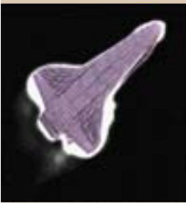
The enhanced image of the plasma field surrounding the Columbia. The wire model of the spacecraft has been inserted to aid perspective
