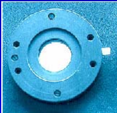
JENOPTIK LC SLM 832 × 624 pixels 30 ms response time
