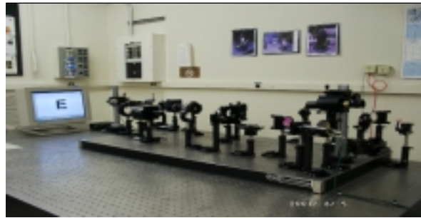
The Liquid Crystal Spatial Light Modulator (LC-SLM) AO system designed by LLNL for delivery to UC Davis. Photograph Scot Olivier, LLNL
