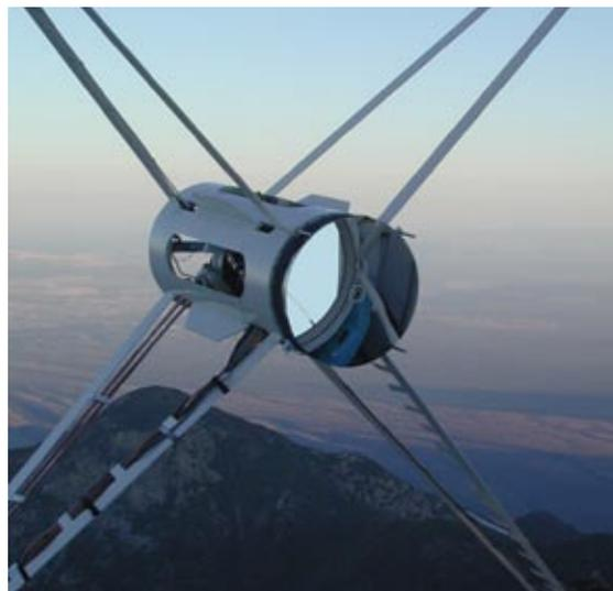
Fig. 2 The Secondary Mirror installed on the 6.5m MMTO telescope.
