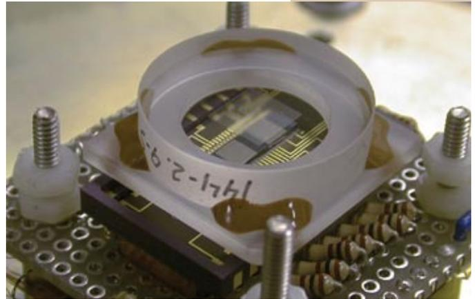
*Fig 5 The Shack-Hartmann wavefront sensor. The lenslet array is just visible as a square patch within the hockey puck shaped glass substrate.*
