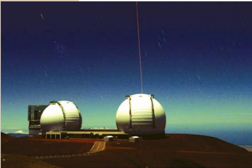
*Fig. 1 The Keck laser creates a high altitude artificial star, allowing the adaptive optics system to measure and correct for turbulence in the Earth's atmosphere. Images taken with adaptive optics have a resolution at near infrared wavelengths that is comparable to optical images taken with the Hubble Space Telescope.*
