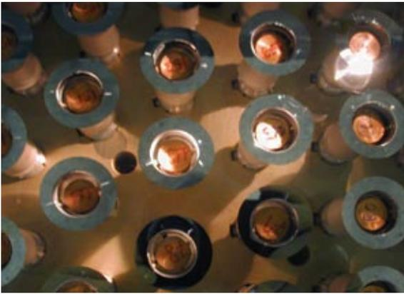
*Fig 4 Looking into the reference body, the capacitance sensors are visible as metal coated rings surrounding the actuator fingers. Through the reference body, the cooling plate can be seen.*
