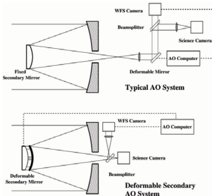
Fig 1 Comparison of the optical layout of the MMT AO system and other AO systems.
