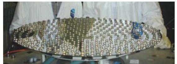
*Fig 3 The Secondary Deformable Shell. The 336 magnets can be seen on the back surface of the mirror.*
